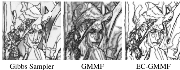
Fig. 3. Maximum value of the marginals: Dark pixels denotes low (high entropy) values.
