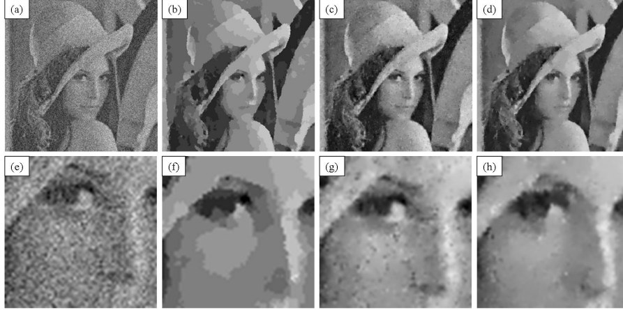
Fig. 5. First row: Explicit entropy control allows us restore images by using estimators other than the MPM (see text). Second row: Details.
