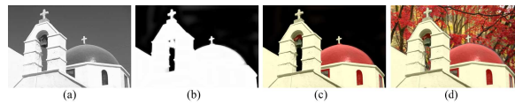
Figure 19: (a) Original image, (b) mask obtained from vector measure field, (c) extracted colored object (d) photomontage using the mask in panel (c).
