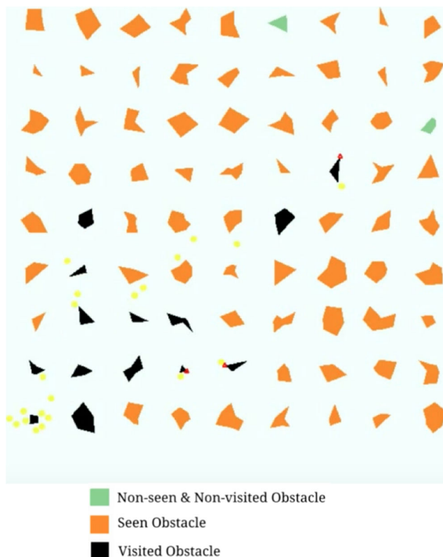
Fig. 20 Exploration of an environment with disc-shaped robots. This experiment is done with 81 distinguishable obstacles and 50 robots
