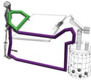
Fig. 8. In the animation phase, two closed kinematic chains are formed between the characters and the object.
