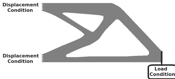
Figure 1.1: Example of structural optimization
