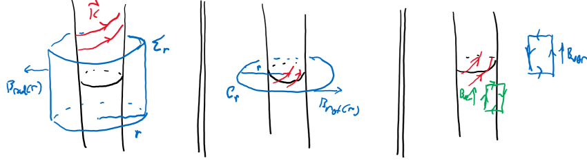
Figure 30. The components of the magnetic field generated by a solenoid may be determined by applying the integral theorems ( \nabla \cdot \vec{B} = 0 , and Ampere's law) to suitable curves and surfaces.
