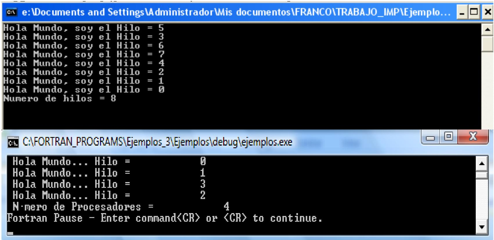
The image shows two screenshots of a Windows command prompt window. The top screenshot shows the output of a program with 8 threads, each printing a message with a thread ID from 5 down to 0, and a total of 8 threads. The bottom screenshot shows the output of a program with 4 processors, each printing a message with a thread ID from 0 to 3, and a total of 4 processors. The program is paused, and the user is prompted to enter a command or press Enter to continue.
