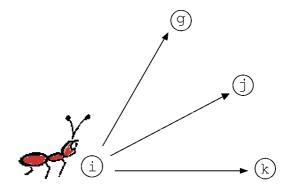
Fig. 2. An ant in city *i* chooses the next city to visit via a stochastic mechanism: if *j* has not been previously visited, it can be selected with a probability that is proportional to the pheromone associated with edge (i, j).
