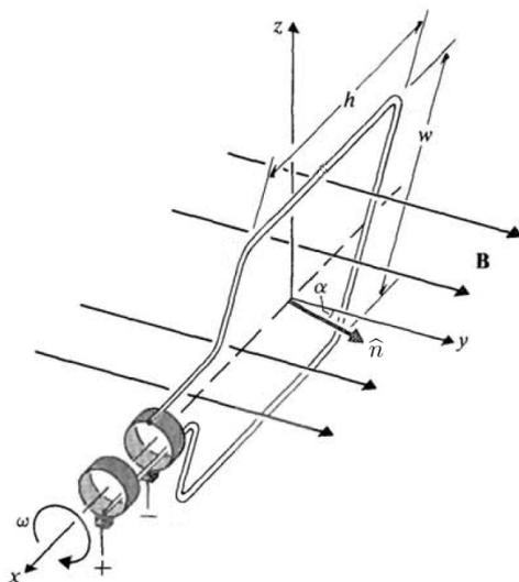
unit normal vector to the loop is  $\hat{n} = \hat{y} \cos \alpha - \hat{z} \sin \alpha$ ,  $\alpha = \omega t$ , the magnetic flux is given by
