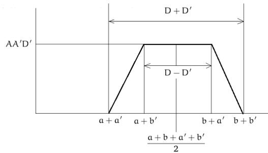
Figure 4: Convolution of two rectangular pulses. ■
