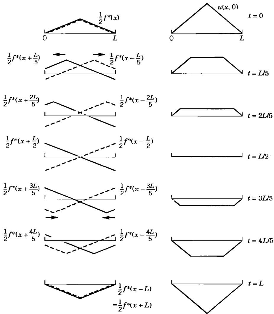
Figure 7: The solution to problem (96), for  $f(z)$  a triangular pulse, and  $g(z) \equiv 0$ . Taken from [20, p. 546].
