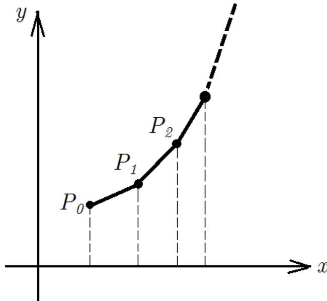
A byproduct of this construction is **Euler's method** to numerically solve the initial value problem
