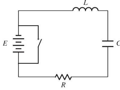
Figure 5: Circuit analyzed in Example 41. Switch is open only on time interval  $[0, 1]$ .
