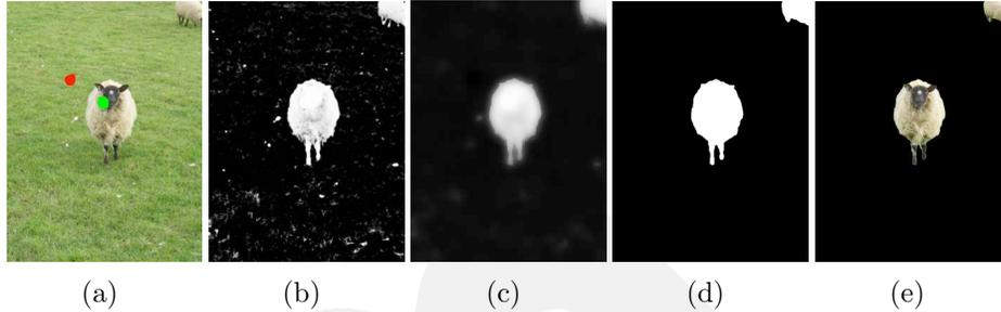
FIGURE 4. Interactive binary segmentation process illustration: (a) Pixels labelled by hand (red and green scribbles), (b) Likelihoods computed from the empirical class distributions, (c) computed  $\alpha$  map, (d) label map (maximum  $\alpha$ ) and (e) segmented image.
