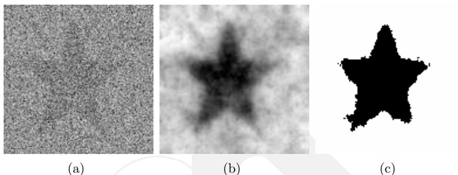
FIGURE 9. Robustness to noise: (a) Synthetic image, (b) computed  $\alpha_1$  and (c) segmentation.
