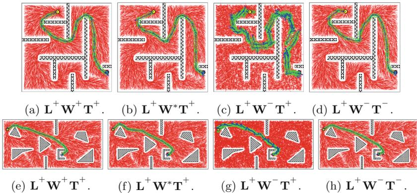
**Fig. 4.** Trajectories generated using the four different local planners for given start and goal states.
