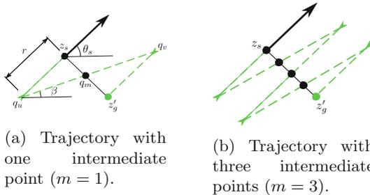
**Fig. 1.** Trajectories (dashed lines) computed by  $L^+W^-T^+$  to reach a state  $z'_g$  from state  $z_s$ .
