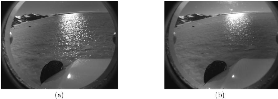
Figure 3. (a) Image without any filter (b) Image with linear polarizing filter.
