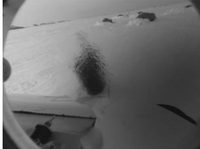
Figure 1. Image with ice on lens
