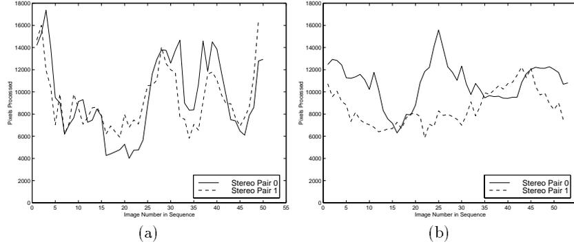
Figure 4. (a) Pixels processed for stereo pairs 0 and 1 while driving in 4.0m radius circle on snow. (b) On blue ice.
