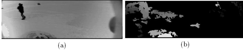
Figure 7. (a) Image of rock on ice. (b) Disparity map. Note the good disparity on the rock (lower middle) and the person, but not the surrounding ice.
